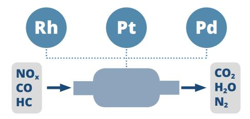
Three-way catalytic converters are present in all petrol-powered cars, and help remove carbon monoxide, unburnt hydrocarbons, and nitrogen oxides. They contain precious metals such as rhodium, platinum, and palladium to accomplish this. Three-way catalytic converters can't be used in diesel engines, as diesel's oxygen-rich exhaust gases make their removal of NO<sub>x</sub> inefficient.
