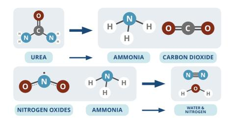
Selective catalytic reduction (SCR) is a method for  $NO_x$  removal that is utilised in some diesel engines. It involves the injection of urea into the exhaust stream of the vehicle, where it is produces ammonia, which is adsorbed onto a catalyst. The ammonia can then react with the nitrogen oxides in the exhaust stream to produce nitrogen and water. SCR is capable of achieving  $NO_x$  reductions of up to 90%.
