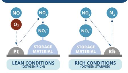
NO<sub>x</sub> adsorbers can also be used in diesel engines. The majority of NO<sub>x</sub> emissions from the diesel engines are NO, and this is converted to NO<sub>2</sub> by reaction with oxygen using a platinum catalyst. The NO<sub>2</sub> is then absorbed in the form of nitrates by the storage material (often barium oxide). Once the trap is full, the nitrate can be desorbed, converted to nitrogen over a rhodium catalyst, and released.
