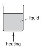
The density of the liquid changes as its temperature increases. This causes energy to be transferred throughout the liquid.
