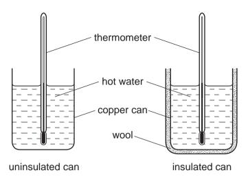
One can is insulated with wool. The temperature of the water in each can is taken every minute for several minutes. Graphs of the results are plotted.
