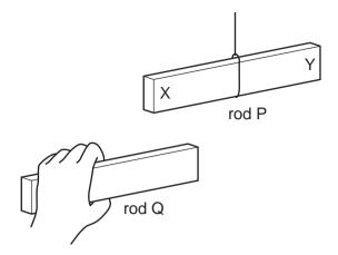
The end of rod Q is brought near to end X of rod P, and then near to end Y of rod P.
