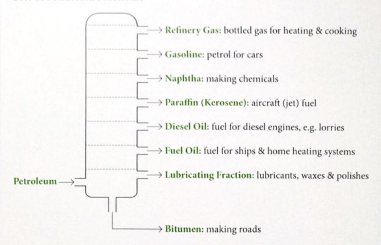
The fractionating tower is hottest at the bottom and coolest at the top
