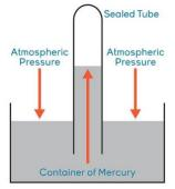
The pressure beneath a liquid surface increases with depth and density.
