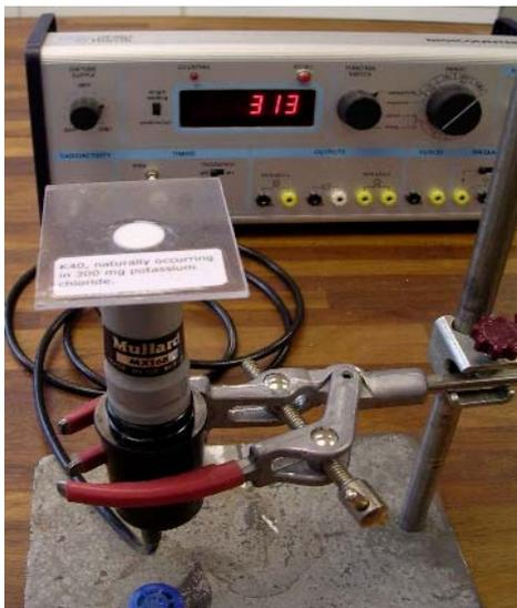
1. Position the GM-tube vertically so the end window is pointing uppermost. Clamp the tube holder, not the tube itself.
