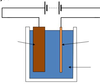
positive pure copper sulphate impure copper electrode battery electrode cathode solution anode electrolyte
